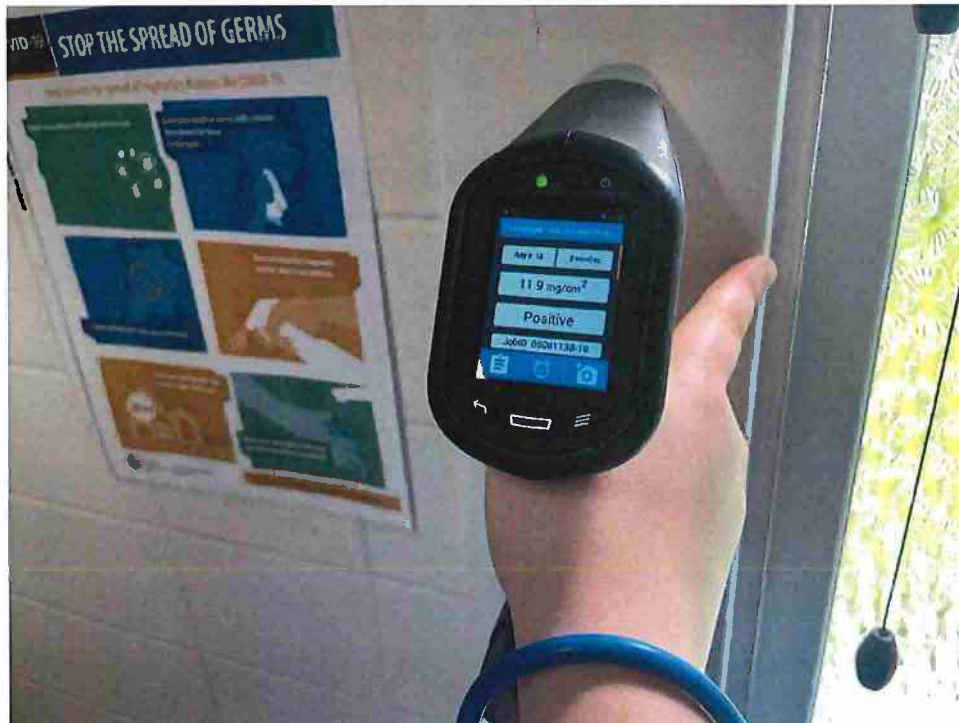
16. View of the white wood tested and identified as Lead-Based Paint
