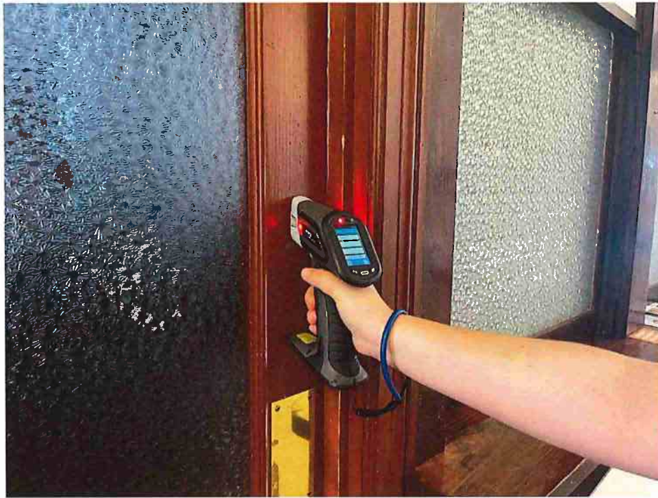
17. Typical view of the brown door components being tested for Lead-Based Paint
